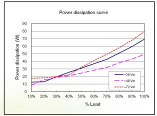
Figure 2: Power dissipation ( $T_A = 25^{\circ}C$ ,  $V_{out} = -54 \text{ V}$ )
