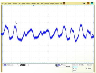
Figure 9: Input reflected ripple current
