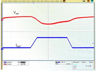
Figure 19: Output voltage dynamic response (load: 10%–90%–10%, di/dt = 0.1 A/ $\mu$ s, T<sub>A</sub> ≥ –25°C)
