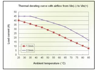
Figure 3: Thermal derating with airflow from Vin (-) to Vin (+) ( $V_{in} = -48$  V,  $V_{out} = -54$  V)
