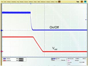
Figure 12: Shutdown from On/Off ( $V_{in} = -48.0 \text{ V}, V_{out} = -54.0 \text{ V}, I_{out} = 44.5 \text{ A}$ )
