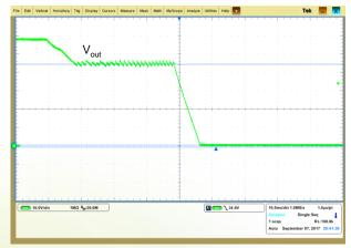
Figure 16: Shutdown from On/Off ( $V_{in} = -72.0 \text{ V}, I_{out} = 20.7 \text{ A}$ )
