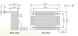
Figure 27: Standard heat sink for airflow from V<sub>in</sub> to V<sub>out</sub>
