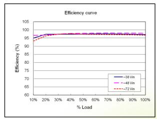
Figure 1: Efficiency ( $T_A = 25^{\circ}C$ ,  $V_{out} = -54 V$ )
