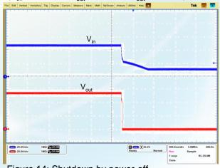
Figure 14: Shutdown by power-off ( $V_{in} = -48.0 \text{ V}, V_{out} = -54.0 \text{ V}, I_{out} = 44.5 \text{ A}$ )
