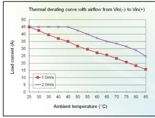
Figure 5: Thermal derating with airflow from Vin (-) to Vin (+) ( $V_{in} = -60 \text{ V}$ ,  $V_{out} = -54 \text{ V}$ )
