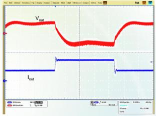
Figure 18: Output voltage dynamic response (load: 50%–100%–50%, di/dt = 1 A/ $\mu$ s, T<sub>A</sub> ≥ –25°C)
