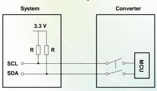
Figure 21: Interconnect diagram of SCL and SDA
